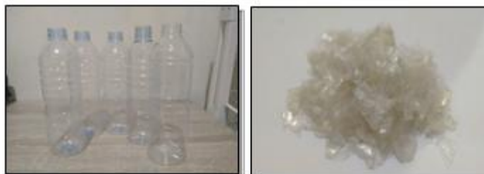
Figure 7: PET Plastic Material before and after Grinding Process.
