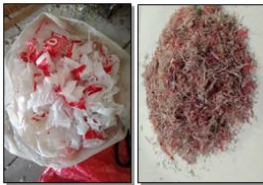
Figure 5: LDPE Plastic Material before and After Grinding Process.
