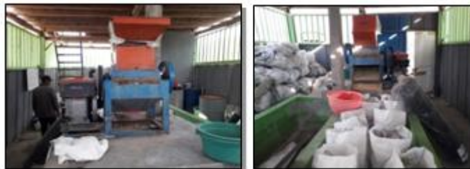
Figure 6: PET Plastic Waste Shredder.
